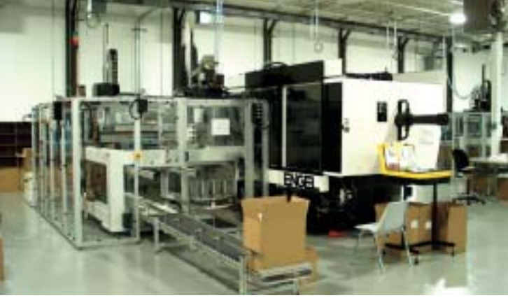
Mar-Lee: In-mold labeling cell consisting of high speed Engel 450 ton toggle machine and ERS (Speedy) servo robot.
