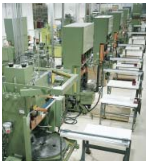
19 vertical presses from 55 through 200 tons run in the third injection molding bay.
