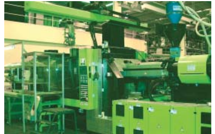
Hague: Three mold changes per week are performed on this 660 ton ENGEL TIEBARLESS machine, equipped with an ERC 74/1-C robot.
