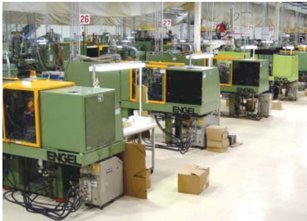
A total of 47 horizontal presses, ranging from 40 to 660 US tons, are located in two of Fabrik's injection molding bays.
