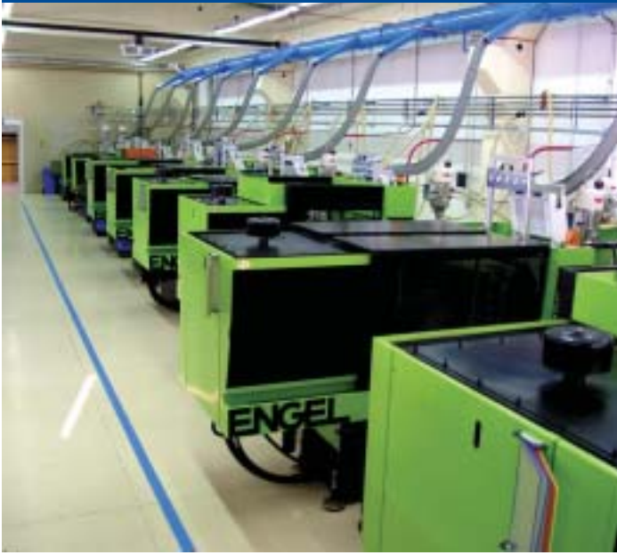
Kovinoplastika Janez Povše s.p.: the new production facility operates ten injection moulding machines, all of them from Engel, with clamping forces ranging from 350 to 1,100 kN. Fifteen employees produce parts for kitchen appliances and hand tools. Some parts are joined together to form complete sub-assemblies using ultrasonic welding (centre photo), a technology in which Kovinoplastika Povše is the specialist in Slovenia. The company processes all common engineering plastics from ABS and POM through to glass strand reinforced PA and, more recently, PEEK. Right-hand photo: Janez Povše (left) is always pleased to see Vojko Rogelj of Lesnik. He appreciates him as a highly competent consultant. One of the current matters under discussion is Kovinoplastika Povše's plan to produce components for medical equipment.
