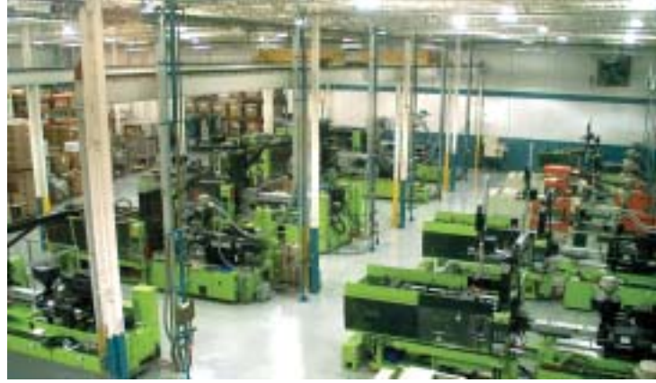
Mar-Lee: The custom molding facility with Engel machines from 22 to 750 US tons.
