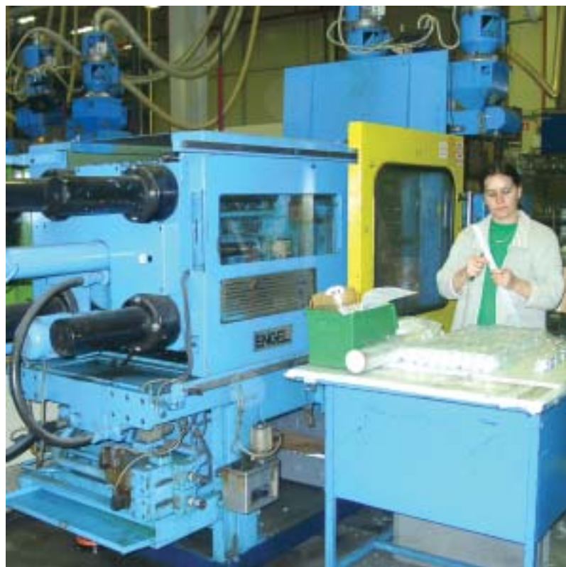
Gorenje has concentrated all its facilities – production, warehousing and R&D – in Velenje. The grounds have a total area of 350,000 m 2 , of which 195,000 m 2 are covered with buildings. The company now operates 30 injection moulding machines, including 23 Engel machines ranging from 900 to 7,500 kN, all of them equipped with robots. The oldest machine, built in 1978 (photo above right), is still working as reliably as ever. Systematic and documented maintenance of all machines and moulds ensures that the machines run to 98% of their capacity at all times. 80% of the moulds are produced in Gorenje's own mould making department, which employs almost 200 people.
