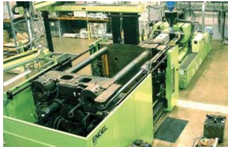
Hague: Brine cabinets and mineral tanks are molded on an ENGEL DUO 1250 with an ERC 84/1-C robot.
