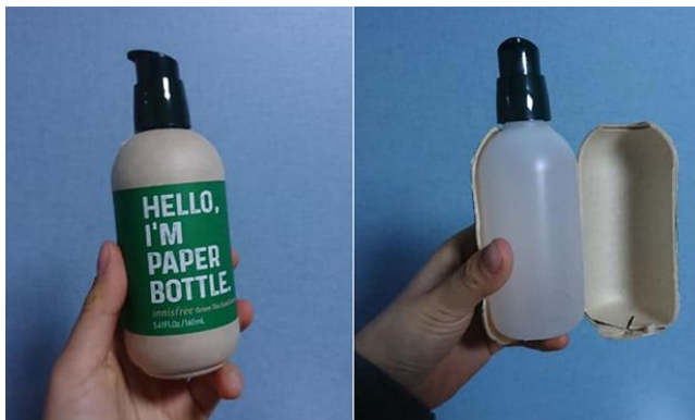
Figure 8: Examples of paper packaging that contain plastic inserts, plastic closures, and plastic pumps
