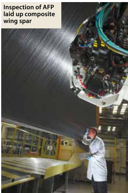
Inspection of composite wing spar section
