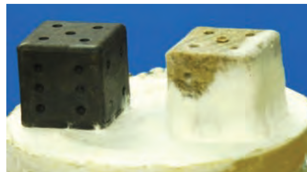
Nerolit/NeroPlast is durable against microbial deterioration.
