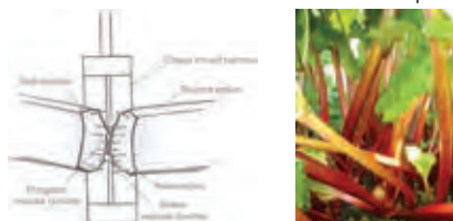
Figure 1: Fracture mechanism of a rhubarb petiole during impact testing
