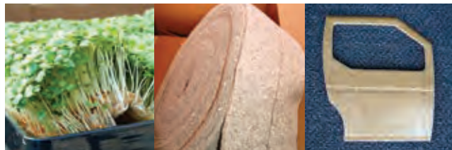
Left to right: Hemp fibre bounded with PLA-fiber a growth medium for spicy herbs, nonwoven hemp fibre mats, reinforced bio-composite. Pictures: Bodil Pallesen.
