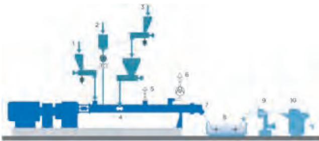
1 Starch / powder premix | 2 Plasticizer / liquid additives | 3 Polymer pellets | 4 Twin screw side-feeder ZS-B | 5 Atmospheric degassing | 6 Vacuum degassing | 7 Die head | 8 Water bath | 9 Airknife | 10 Strand pelletizer
