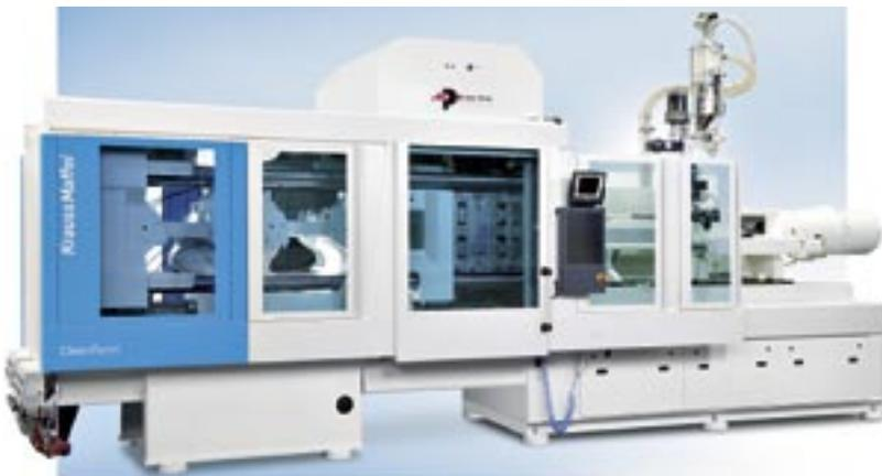
EX injection moulding machine for cleanroom production.
