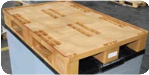
The Injection Moulding Compounder (IMC), developed by KraussMaffei, combines the benefits of injection moulding and extrusion. The manufacture of pallets from filled HDPE illustrates the potential savings achievable with this technology.
