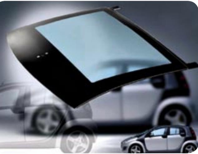
Lower weight and completely new prospects for creating new shapes give plastic a clear edge over glass in many areas of glazing. KraussMaffei's MX SpinForm system is designed specifically for compression moulding these very large parts.
