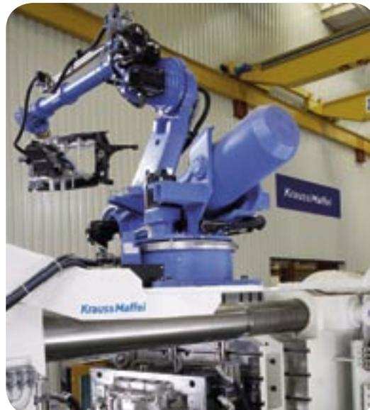
IR industrial robots are the solution to automating large injection moulding machines.
