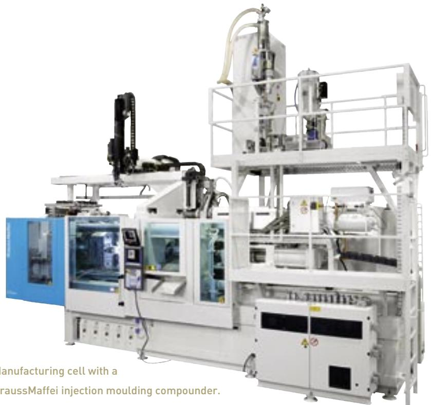
Manufacturing cell with a KraussMaffei injection moulding compounder.
