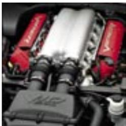
Top performance: each cylinder in the V10 engine has its own individual throttle valve in a plastic housing.
