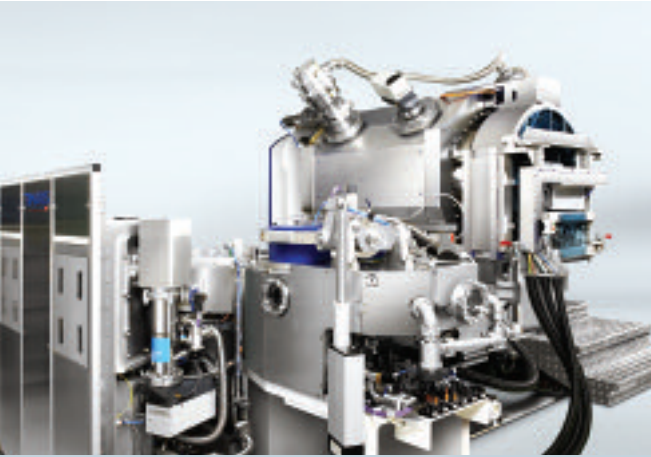
TIMARIS Coatingsystem for Read-Write-Heads and MRAM wafer
