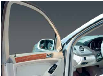
The door-frame finisher of the M-Class Mercedes offers esthetic advantages as well as a reduction of external noises. The multimaterial sealing applications, which have been newly defined as strategic products by Sarnamotive Division America, could already be extended satisfactorily in the past 12 months.
