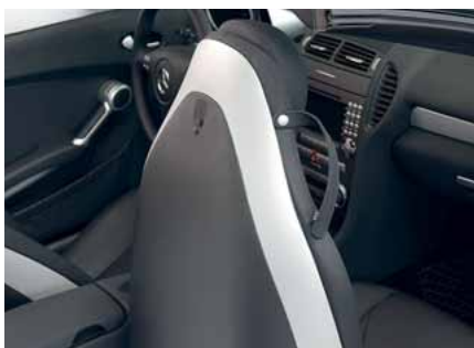
The seat covering of the Mercedes SLK, consisting of plastic and aluminum, provides a high-quality visual effect and stable back support. With this development, Sarnamotive Schenk is responding to the ever more complex requirements of modern vehicle interiors.
