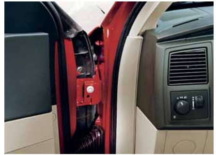
The sealing of the passenger compartment of the Dodge Ram reduces the wind noise in the passenger compartment. The design concept of the multimaterial sealing, originally developed for the Chrysler 300M, was successfully transferred to other Chrysler platforms.
