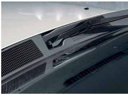
The cover of the Mitsubishi Galant installed between the hood and windscreen draws fresh air into the vehicle's interior and prevents fouling of the heating, air-conditioning and ventilation module.
